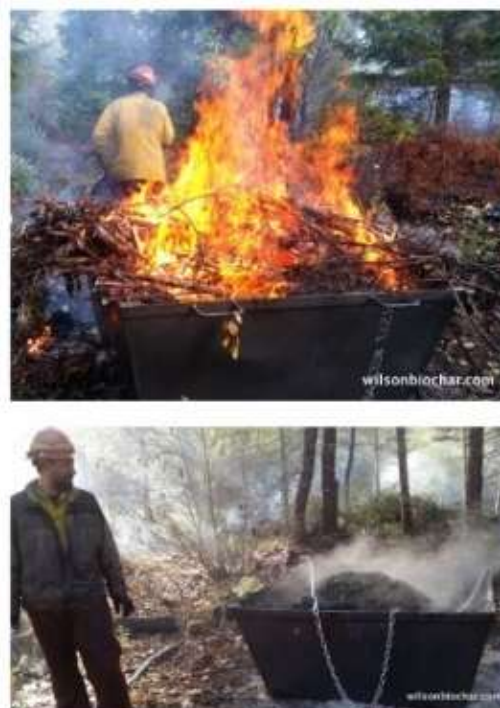
Figure 15. The Forestry Flame Cap Kiln. Designed by Wilson Biochar Associates for use in forestry to convert burn piles to biochar. Newer model will have fork pockets for lifting and unloading. Biochar for Forest Restoration in the Western United States – 9-18-15 (rev.3-15-16)
